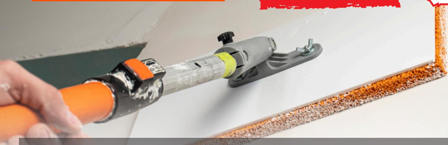
**CEILING SPONGE FLOAT** is designed to finish grainy surfaces such as sand and cement mix, or for applying certain plaster finishes. Coarse sponge rubber pad with a thickness of 18 mm enables easy removal of dirt, and at the same time, thanks to its porous structure, keeps water in it. The swivel attachment allows the work with an extension pole, thanks to which access to hard-to-reach places such as high walls or ceilings will be much easier.
